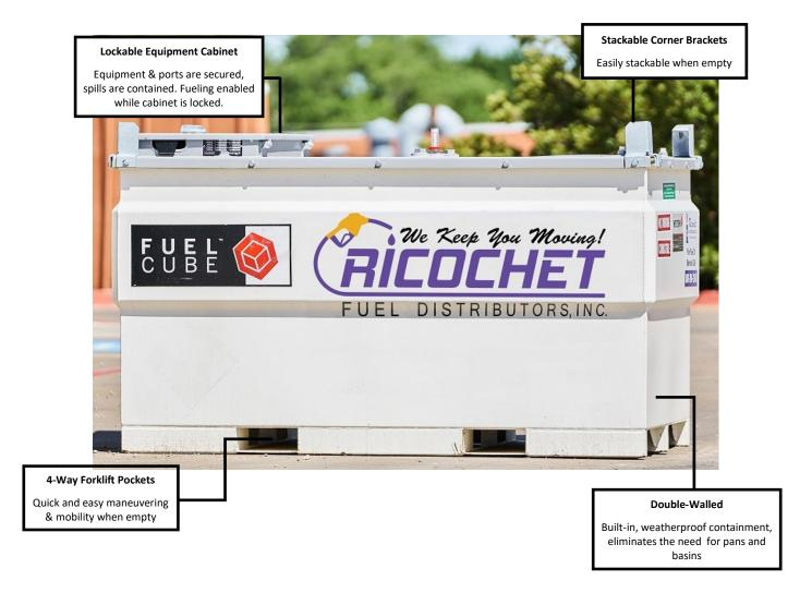
The FuelCube is a double-walled stationary fuel tank built for onsite equipment refueling and backup fuel supply. Fuel Cubes offer increased portability and security over standard bulk tanks. With an included pump, lock box, and containment system, Fuel Cubes provide you with an all-in-one fuel storage solution for your jobsite or yard.
